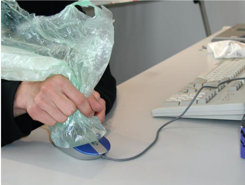
Fig. 5. Reactivating a latent image can also be done with a little water in a plastic bag.
