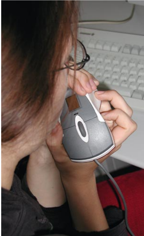
Fig. 3. Even simple breathing will do the trick of outwitting a capacitive fingerprint scanner.
